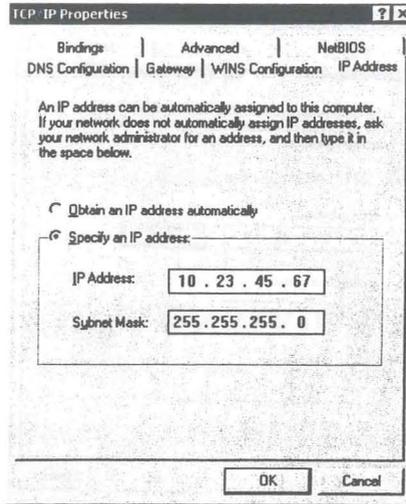
**IP-Address tab:** Choose **Specify an IP address**. Enter your IP address (can be found on the piece of paper at the end of your table), and the subnet mask (255.255.255.0)
