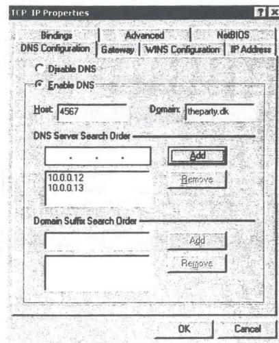
**DNS Configuration tab:** Choose **Enable DNS**. The **Host** field should be the last two octets in your IP number. (If your IP is 10.23.45.67 then the hostname should
